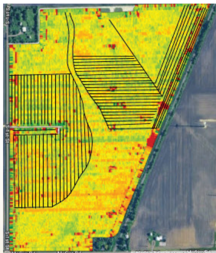
Yield map before and after: Red zones on the left map reflect low yields from excessive water. Drainage tile was selectively installed in these wet areas (black lines in the right image), leading to higher, more consistent yields.
